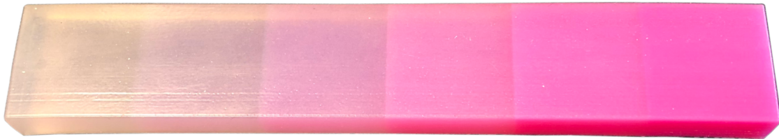
Figure 21: Image of the sample used in the 2/22/2021 run of Test D. The portions that are more translucent contain more Agilus30, while the sections that are more pink contain more VeroVivid Magenta. The target hardness values for each unique material combination are {40,50,60,70,85,95} (left to right).
