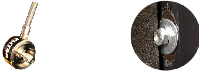
Figure 27: A picture of the LCM300 load cell (left) and its experimental setup, as seen from the inside of the black box enclosure (right).
